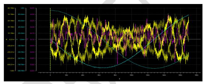
As discussed in previous chapters on the left part are displayed the references vertical axes, one for each different measurement unit of the displayed waveforms. Each axis has its own dynamic range that can be tuned by using the magnitude and offset spinners described in previous chapters.
