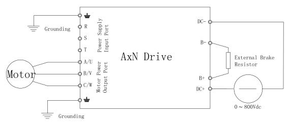
**Main Circuit Connection Diagram: DC Power**
