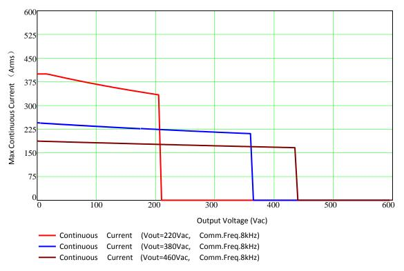
CONTINUOUS AND PEAK CURRENT VS OUTPUT VOLTAGE AT 40  $^{\circ}\mathrm{C}$  AMBIENT
