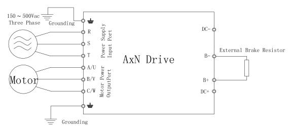
**Main Circuit Connection Diagram: AC Power**
