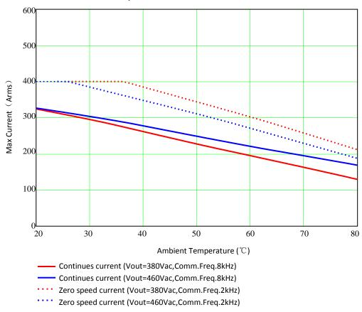
MAX CURRENT VS AMBIENT TEMPERATURE
