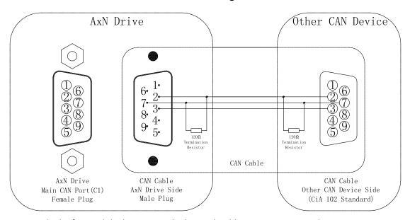
Note: Only the first and the last CAN node device should use a  $120\Omega$  terminal resistor.
