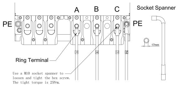
**Motor Power Output Cable Installation**
