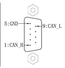
Note: CANOpen pin assignment on S1 connector does NOT meet CiA 102 Standard.
