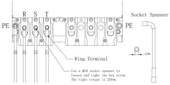
**AC Power Supply Cable Installation**
