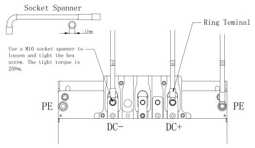
**DC Power Supply Cable Installation**
