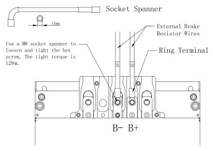
**External Brake Resistor Installation**
