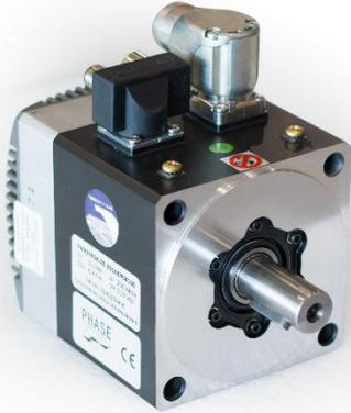
The TorqueWire motor system consists of an advanced, high performance rare earth brushless servo motor, a DSP based, high voltage interpolating servo drive and a single or multi turn absolute encoder, all assembled in a very compact IP 65 protected frame. The motor systems are controlled via a EtherCAT or CANopen fieldbus, linking together groups of motors on a single bus system
