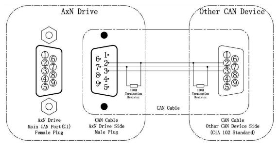
Note: Only the first and the last CAN node device should use a  $120\Omega$  terminal resistor.
