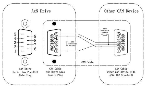
Note: Only the first and the last CAN node device should use a  $120\Omega$  terminal resistor.
