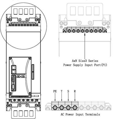
**Step 4: Insert Wires into Corresponding Terminals**
