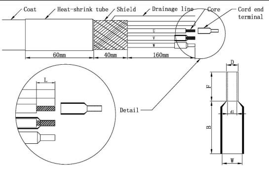
Step 7: Connect the PE wire with Shield
