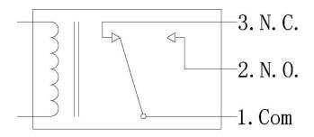
When the drive is ready, N.O. connects Com and N.C. disconnects Com, illustrated as below.
