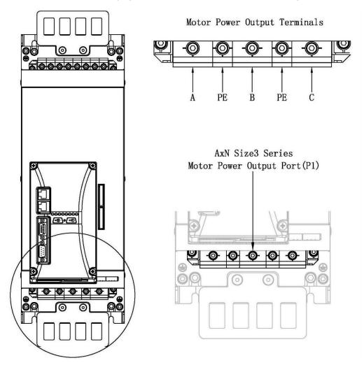
Step 2: Insert Wires into Corresponding Terminals
